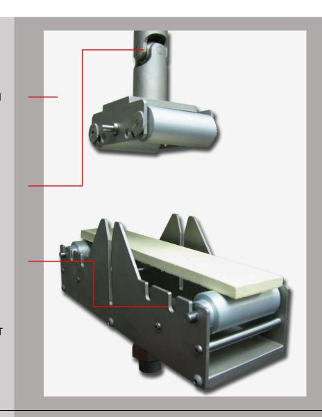
Easy to use winTest Analysis software included, pre-programmed with GRC test parameters (EN 1170-5, GRCA MOT Part 3)
