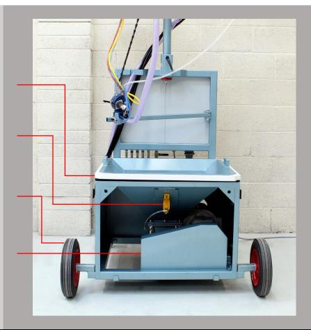
Heavy duty spring easily supports the weight of the boom, gun and hoses
