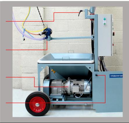
Material sieve to filter large cement particles, reducing blockages
